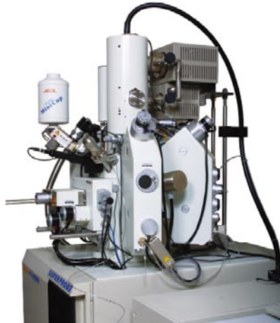
電界放射型電子銃を装着した波長分散型EPMA EPMA (electron probe micro analyzer) equipped with wavelength dispersion spectrometers and the thermal filed emission electron gun.
